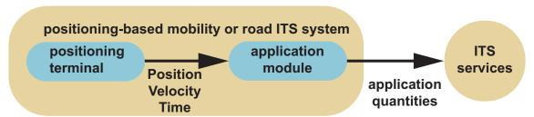
For instance, the system Personal Navigation Device (PND) comprises a positioning terminal (the GNSS receiver chipset with its antenna) and an application which performs map-matching, attributes retrieval and user information generation through the human-machine interface. The service is the guidance to the driver.
