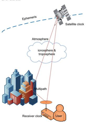
The frequency band allocated to Radio Navigation Satellite Service (RNSS) is the L-band, in particular its upper (1559-1610 MHz) and lower (1151-1214 MHz) parts. Each satellite transmits signals at two or three frequencies in the L-band that have three main components: ranging code, carrier phase and navigation message.
