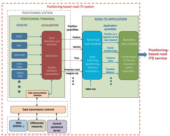
A GNSS-based positioning terminal, potentially merging other sensors or sources of data, provides a position (3D, 2D or 1D) expressed in an absolute reference system, such as WGS84. However, depending on the processing done in the terminal and the chosen data stream, it can also provide velocity (3D or 2D vector), speed (the magnitude
